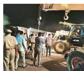
Truck being straightened with the help of JCB and crane.
